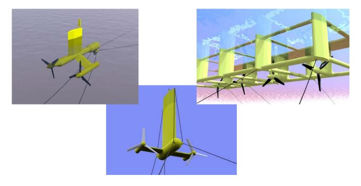
The turret moored solutions are used with Oceanflow's in-house fixed pitch turbine design while the spread moored solution employ third party OEM's variable pitch turbines.
